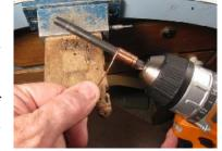
screw gun chuck. Then wind slowly, keeping a tight coil. I like to rest the end of the mandrel on the edge of the table or bench pin. Finally, one note of caution. If you are winding an entire length of wire, be careful as you get near the end of the wire. If the end passes under your thumb, it can cause a nasty scratch or cut.
