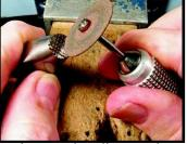
The tool I like to use to grind the pattern is a thin separating disc in a Foredom or Dremel. Be sure to hold the hammer
