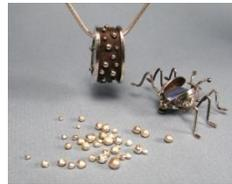
If you need to make all the balls the same size, you need the same amount of metal to melt each time. The best way to do that is to clip equal lengths of wire.
