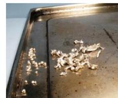
grab your tweezers and pick out the ones you need. When you need larger quantities of balls, pour the casting grain out onto a baking pan, tilt the pan a bit, and let all the round pieces roll to the bottom. Bag
