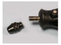
switch collets to use different shaft sizes (3/32- or 1/8-inch bits), and you can't use ordinary drills at all - only the special ones that have a 3/32 shaft.
