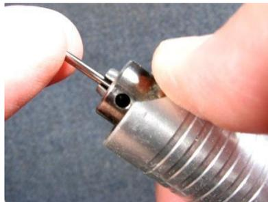
For closing the jaws around a smaller shaft, there's a neat trick. Hold the new bit in the center of the open jaws of the chuck, put your thumb lightly onto the outer toothed collar of the chuck, and gently start up the Freedom. As the chuck turns, it will naturally tighten the jaws around the bur shaft or the drill bit. Then all you have to do is a final tightening with the key.
